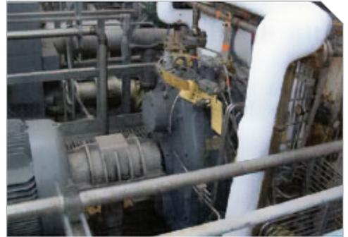
Shown is a Rotoflow mixed gas expander with a speed reduction gearbox.
